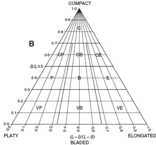
FIG. 5.4 – Diagramme de Sneed et Folk. 10 classes: C (compact), CP (compact-platy), CB (compact-bladed), CE (compact-elongate), P (platy), B (bladed), E (elongate), VP (very platy), VB (very bladed), VE (very elongate)
